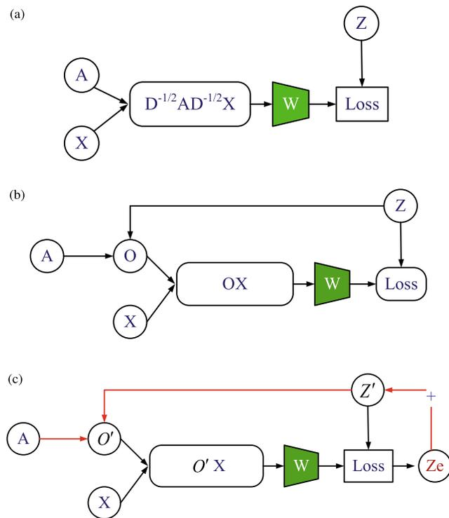
**Fig. 1** The comparison between GCN, TO-GCN, and our proposed E-GCN. GCN adopts the designated topology and feature  $X$  as input to learn the parameters  $W$ . TO-GCN exploits the given labels to participate in learning. E-GCN concurrently learns the  $W$  to comprehensively explore the given labels and estimated labels
